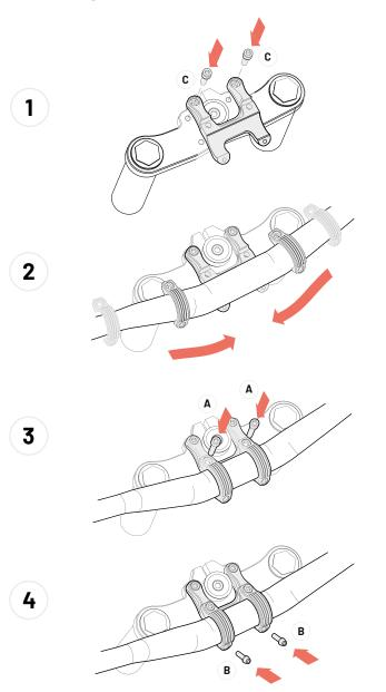
Clean and degrease the clamping surface of the handlebar and stem.
